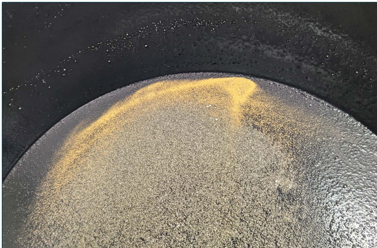
FIGURE 1: GOLD RECOVERED FROM A KNELSON CONCENTRATOR AT 300UM GRIND SIZE (PHOTO CREDIT: IMO).
