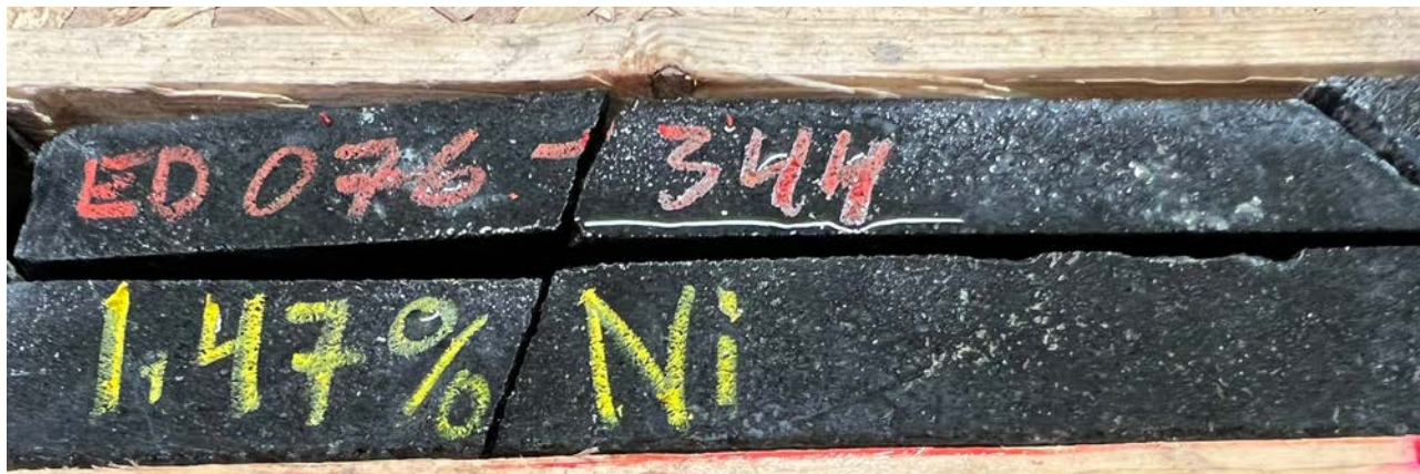
Figure 6: DDED21-076- Drill core sample 344, 1.47% Ni at 332.66m
