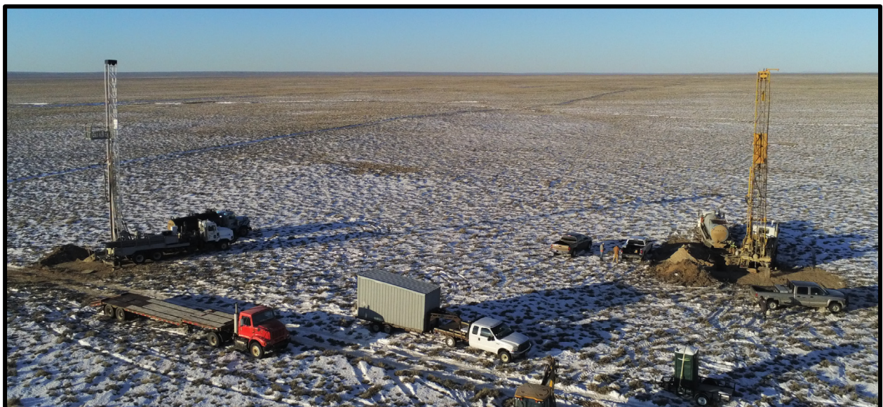
Figure 1. Mud Rotary Drill Rigs Operating at the Thor ISR Uranium Project, GDB, Wyoming USA.
