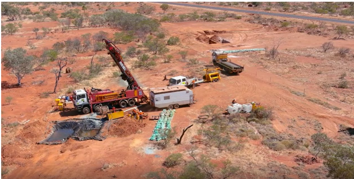
Image 2 - AKN diamond drilling activities at Sandiego.
