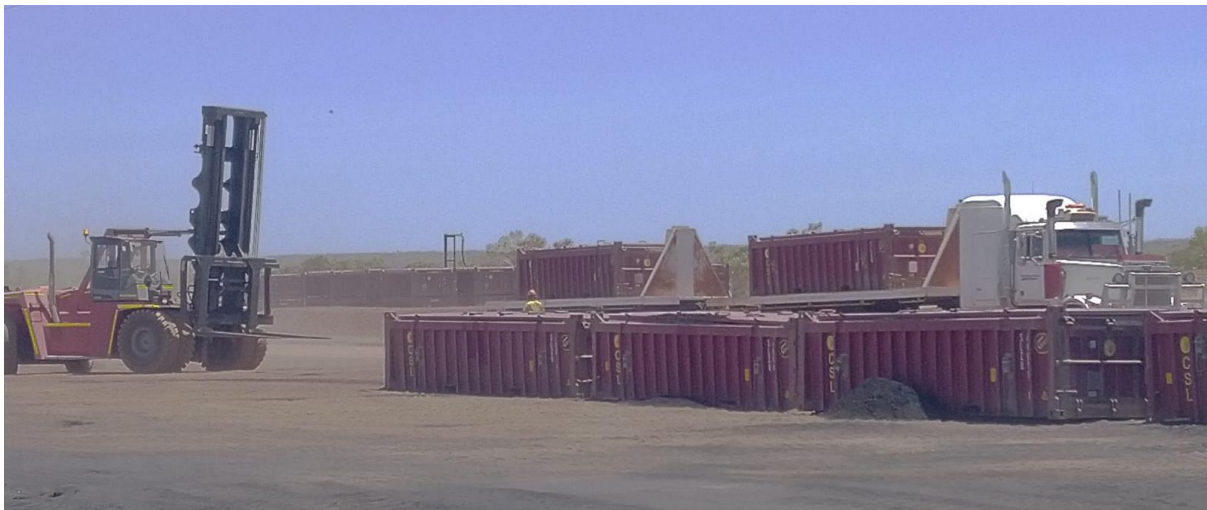
Containers of Magnetite being loaded onto truck for transport to rail siding approx. 20km away
