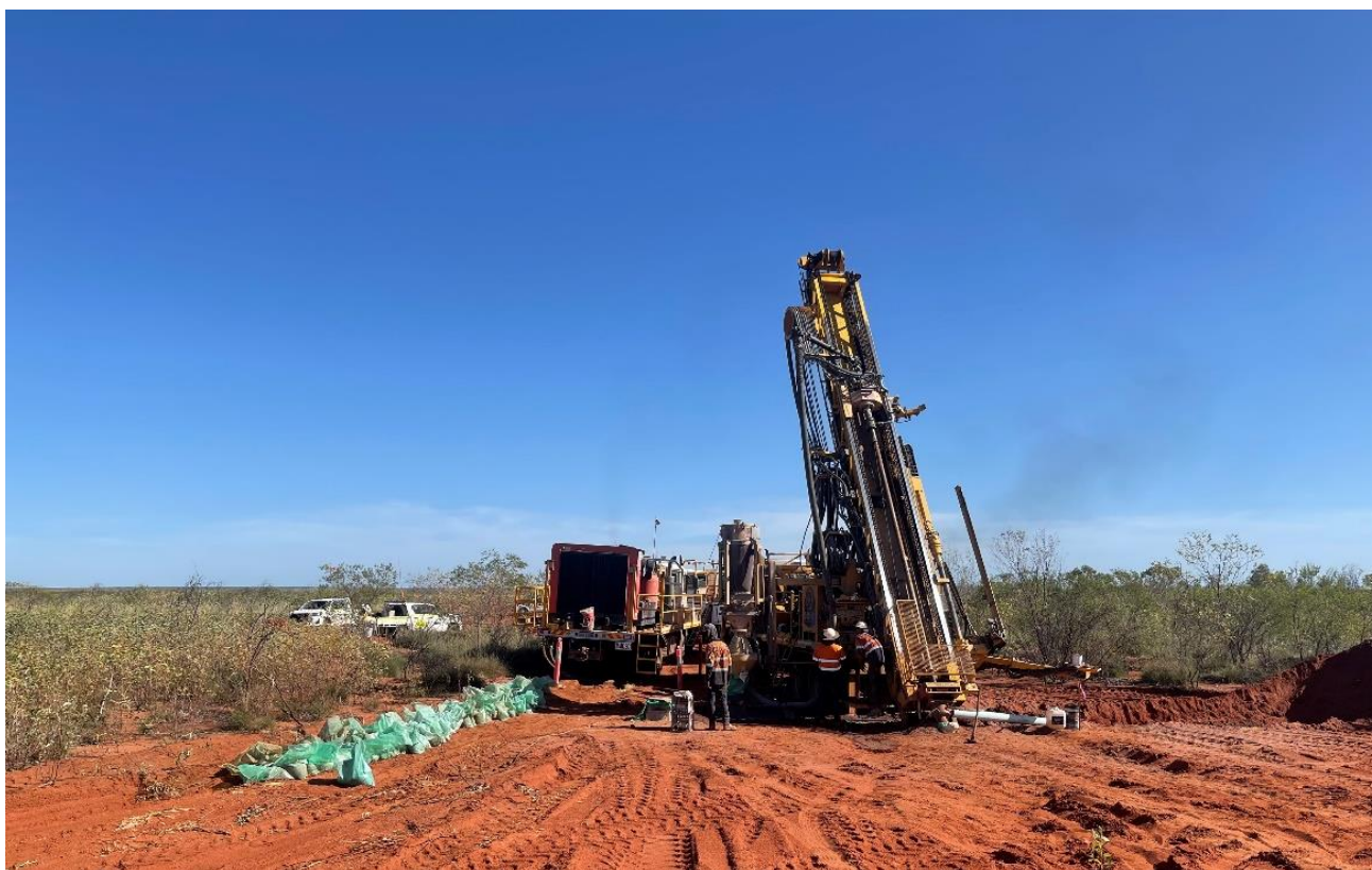
Figure 1: RC drill rig completing the first hole (CPRC001) at the Company's Pardoo Nickel Deposit.
