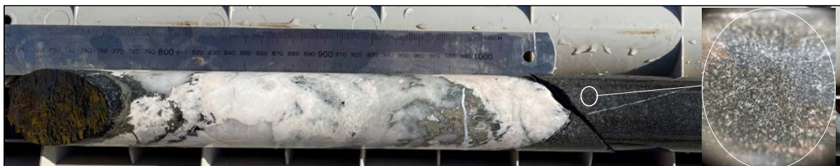
Figure 15: GDRCD007 - 538m, example of quartz-calcite vein in altered diorite with abundant pyrite± chalcopyrite-chlorite-actinolite infill. Close up example of disseminated inter-matrix sulphides in altered diorite.
