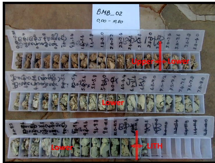
Figure 11: Chip-tray of auger hole BMB_02. This chip-tray clearly illustrates the redox zonation of the Upper sedimentary unit (UpU) into the Upper clay and Lower clay.
