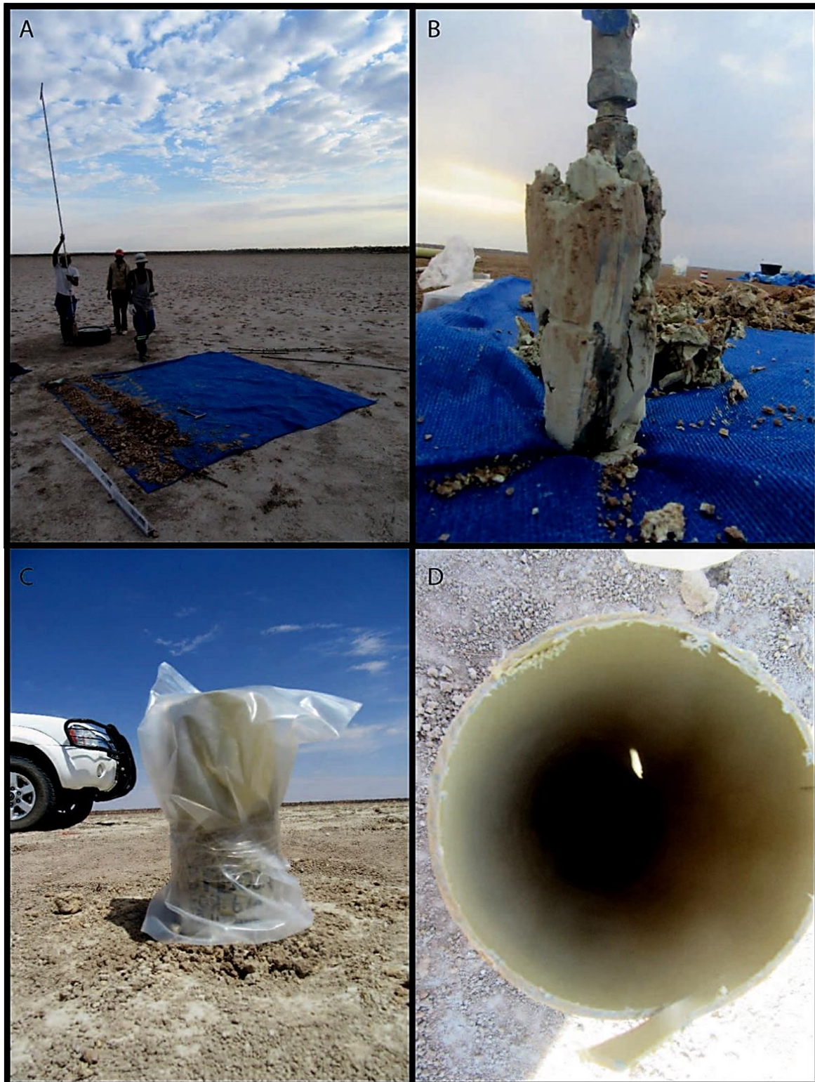
Figure 10: A – Photo mosaic of one of the drill sites, with recovered sediment sample being packed neatly on the canvas cloth as 20 cm samples. The chip-tray sample would immediately be collected and logged. B –The hand auger clay-bit together with its 20 cm interval sample. C – The collar casing which was installed at each drillhole. D – down-the-hole view of one of the drillholes, clearly indicating that the holes remain intact and stable after drilling.
