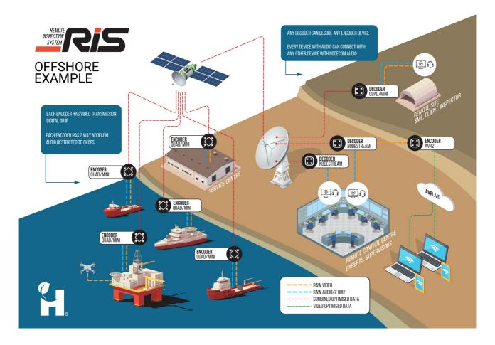
Using HTG's proprietary protocols, RiS™ delivers high-fidelity video, synchronised data, and high-quality audio transmission from any site to another via a secure Local Area Network (LAN).
