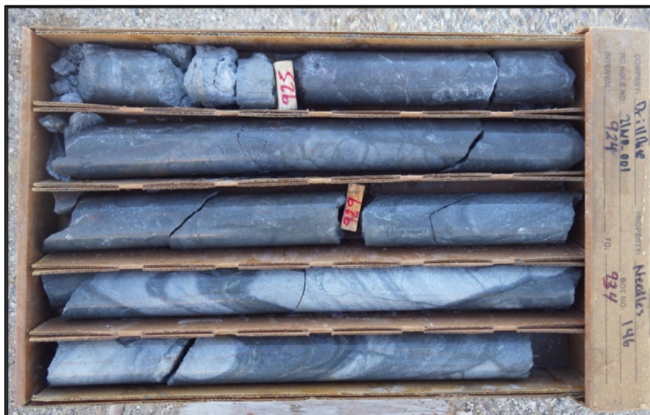
Figure 3. Core photo from 924ft to 934ft (281.6m to 284.7m) in hole 21ND_001 showing silicified and propylitically altered andesites containing disseminated and vein-hosted pyrite (dark grey).
