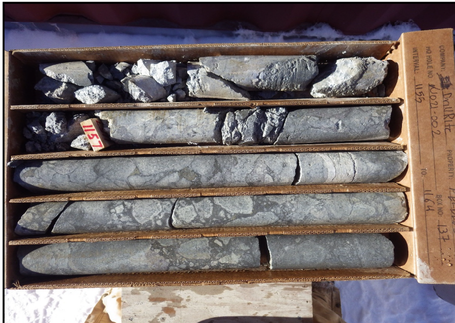
Figure 4. Brecciated unit in hole 21ND_002 showing altered andesite clasts within a pyrite-rich matrix (from 1155 to 1164ft (352 to 354.8m))
