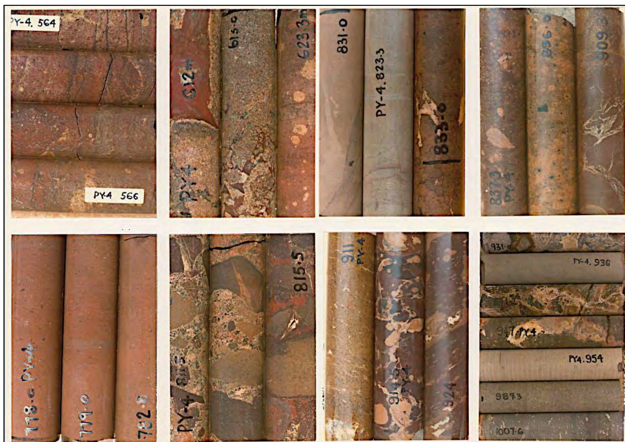
Figure 50: Various GRV rock textures and alteration in PY4
