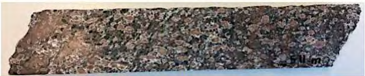
Dacite sill with adularia rims occurring in the GRV @ 511 - 514m
