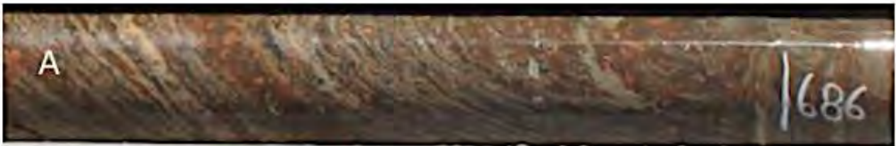
Weakly altered (K feldspar - hematite) porphyritic rhyolite @448.4m
