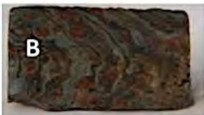
Flow foliation in rhyodacite @686.5m; K-feldspar phenocrysts in devitrified sericitised quartz-plagioclase matrix.
