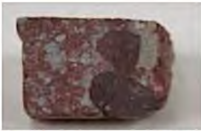
Hematitised microgranophyre pebbles in a sedimentary with disseminated carbonate @429.6m
