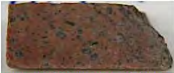
Weakly altered (K feldspar - hematite) porphyritic rhyolite @448.4m
