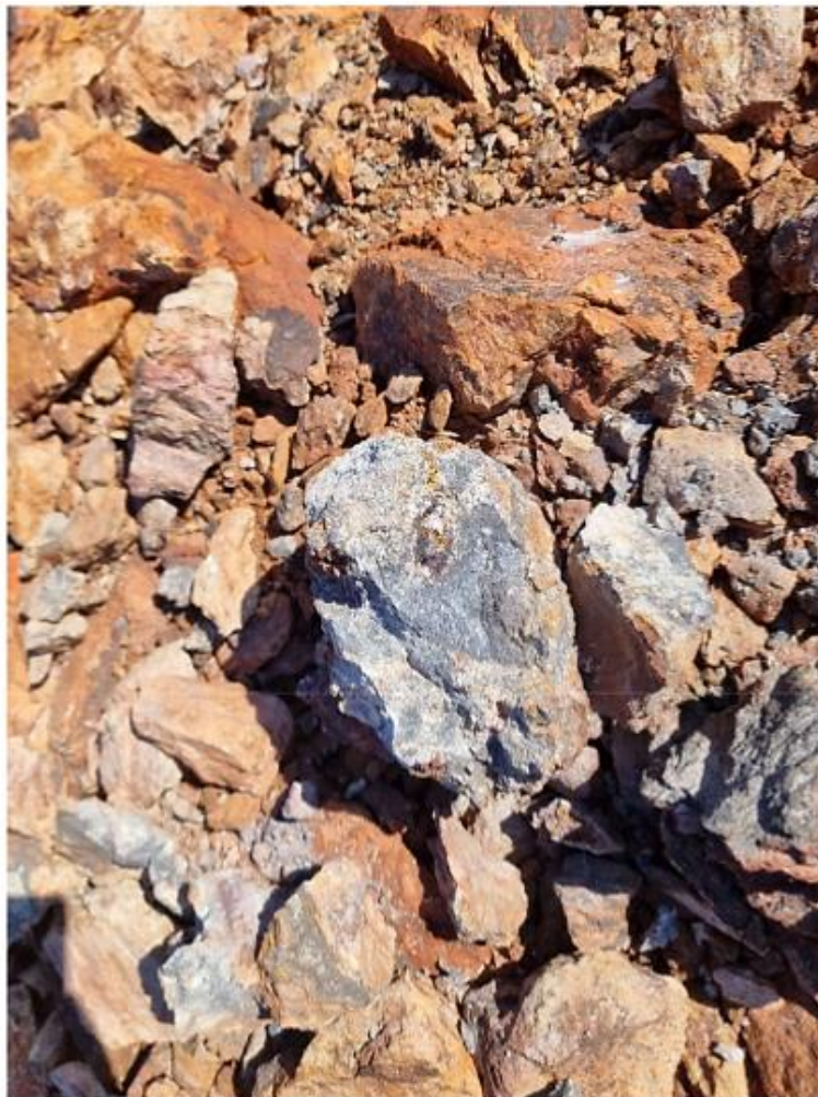
Figure 8 – Highway Prospect showing high grade galena (grey colour) in chert and quartz. The rock in the centre is about fist size.
