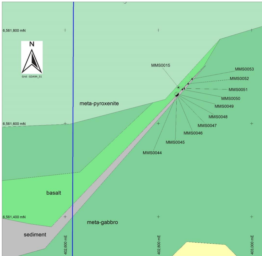
Figure 1: Plan of ten new surface rock-chip sample locations anomalous in copper and zinc
