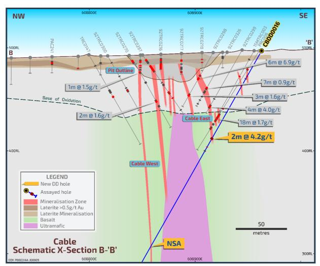
Figure 3. Cross section illustrating mineralisation within RC drill hole CBDD0016.
