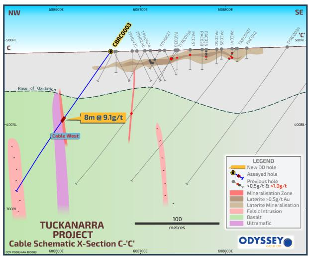
Figure 4. Cross section illustrating mineralisation within RC drill hole CBRC0003.
