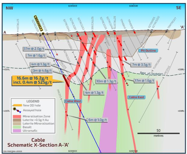
Figure 2. Cross section illustrating mineralisation within diamond drill hole CBDD0023.
