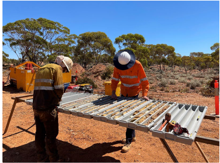
Figure 2 – Drilling the first diamond hole at La Mascotte on 17 March 2022 (left) and examining core from the oxide zone (above)
