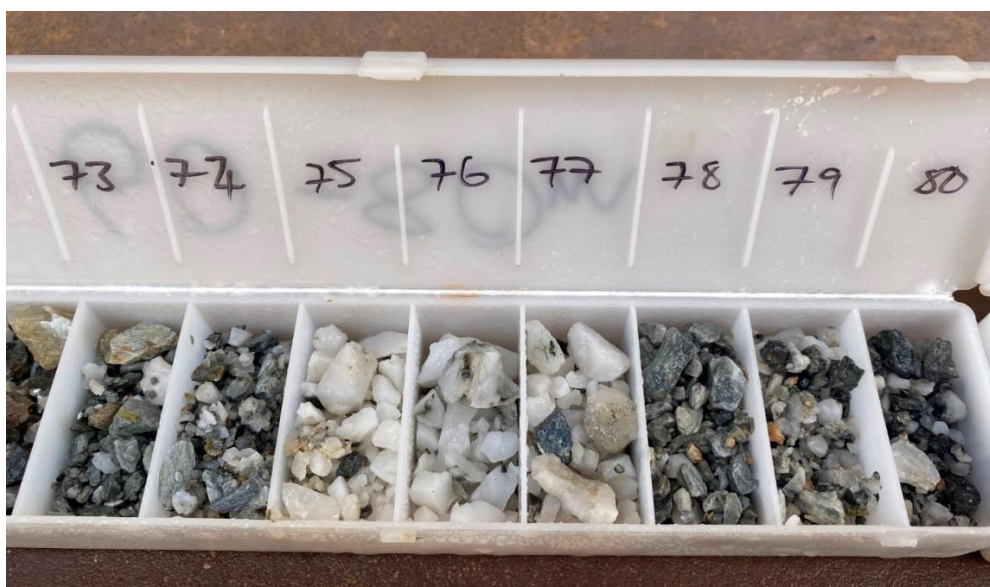
Figure 2. Photograph of RC drill chips from RD21008 (72 – 80 metres) showing quartz veining and sericite ± chlorite alteration
