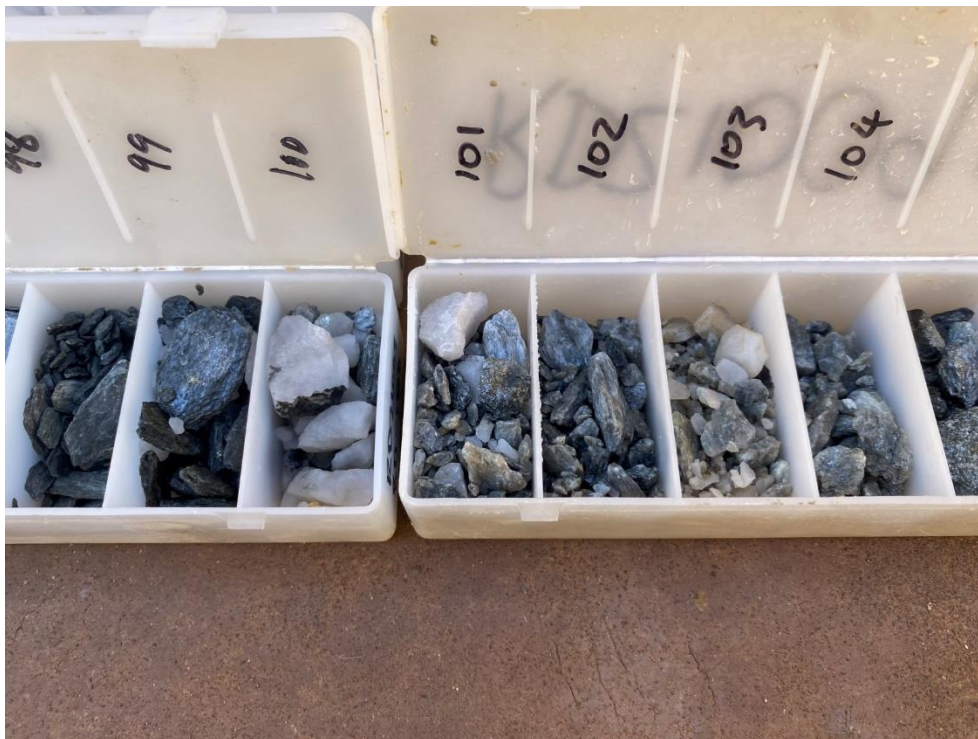
Figure 1. Photograph of RC drill chips from RD21009 (97 – 104 metres) showing visible sulphide and quartz veining present
