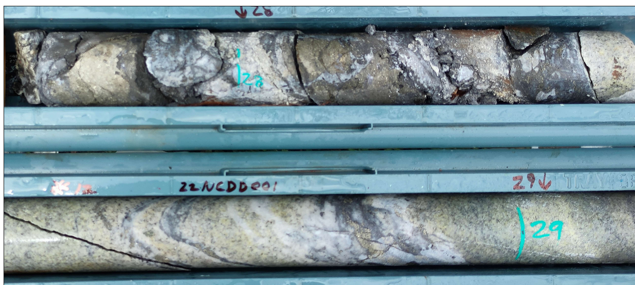
Figure 3. Sulphide-rich mineralised position in diamond hole 22NCDD001 (28m - 29m).
