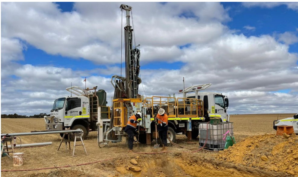
Figure 1: Diamond drilling rig setting up on site at Cloud Nine
