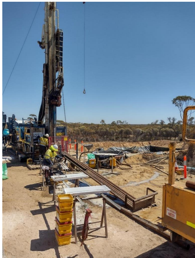
Figure 1. Diamond Drilling in progress at the Boomerang Kaolin Prospect
