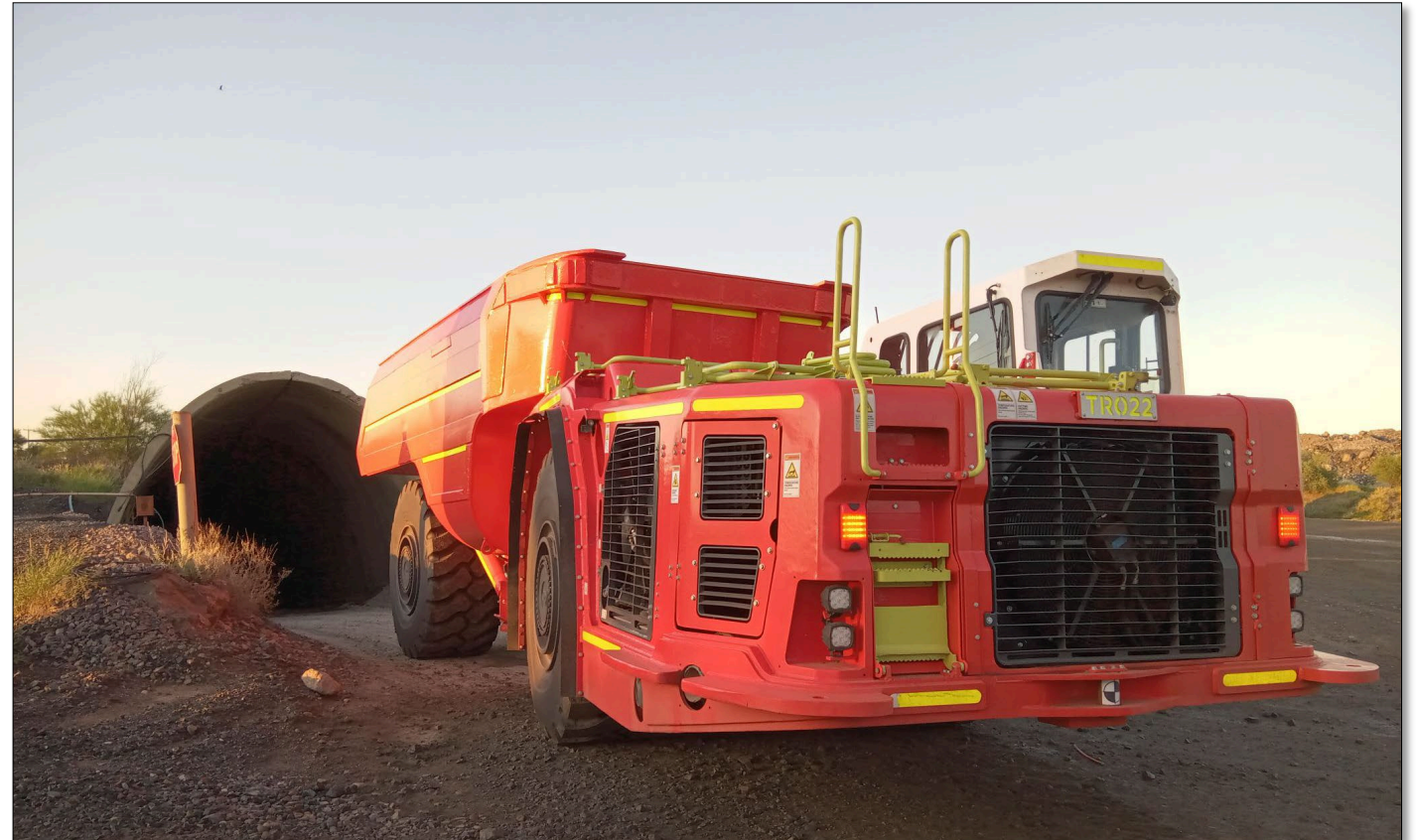
Truck 22 (Sandvik TH663) after a mid-life rebuild February 2022
