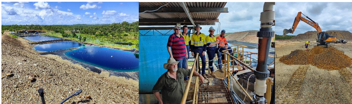
Figure 2 – 2(a) PLS ponds containing residual copper, 2(b) metallurgical and electrical team on site with R3D personnel, 2(c) Sampling the heap leach material to upgrade the resource status and conduct further metallurgical test work.
