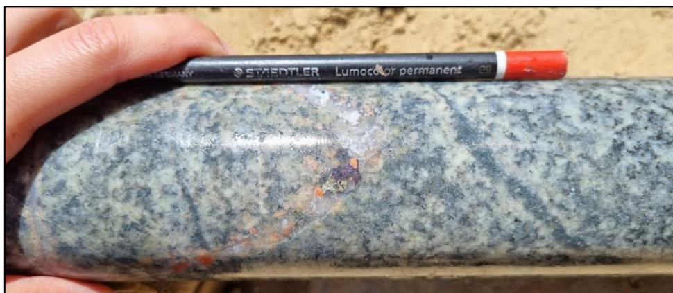
Photo 12. Pyrite-chalcopyrite-bornite (purple) in quartz vein, in tonalite - STWD007 at 453.3m.
