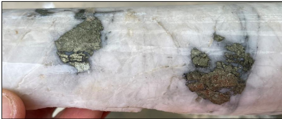
Photo 2. Quartz vein with massive milky white quartz and large chalcopryite chunks - STWD005, 274.2m – 0.6m @ 4.27g/t Au, 0.31% Cu, 2.6g/t Ag and 130ppm Mo.
