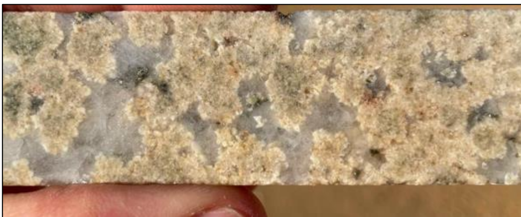
Photo 5. 'Brain rock' unidirectional solidification texture - STWD006, at 108.3m.
