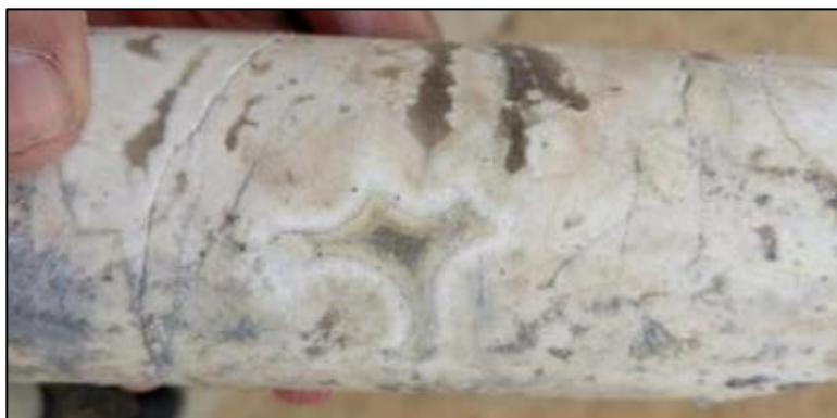
Photo 8. Late-stage cooler dolomite vein with growth textures - STWD006 at 136.7m.
