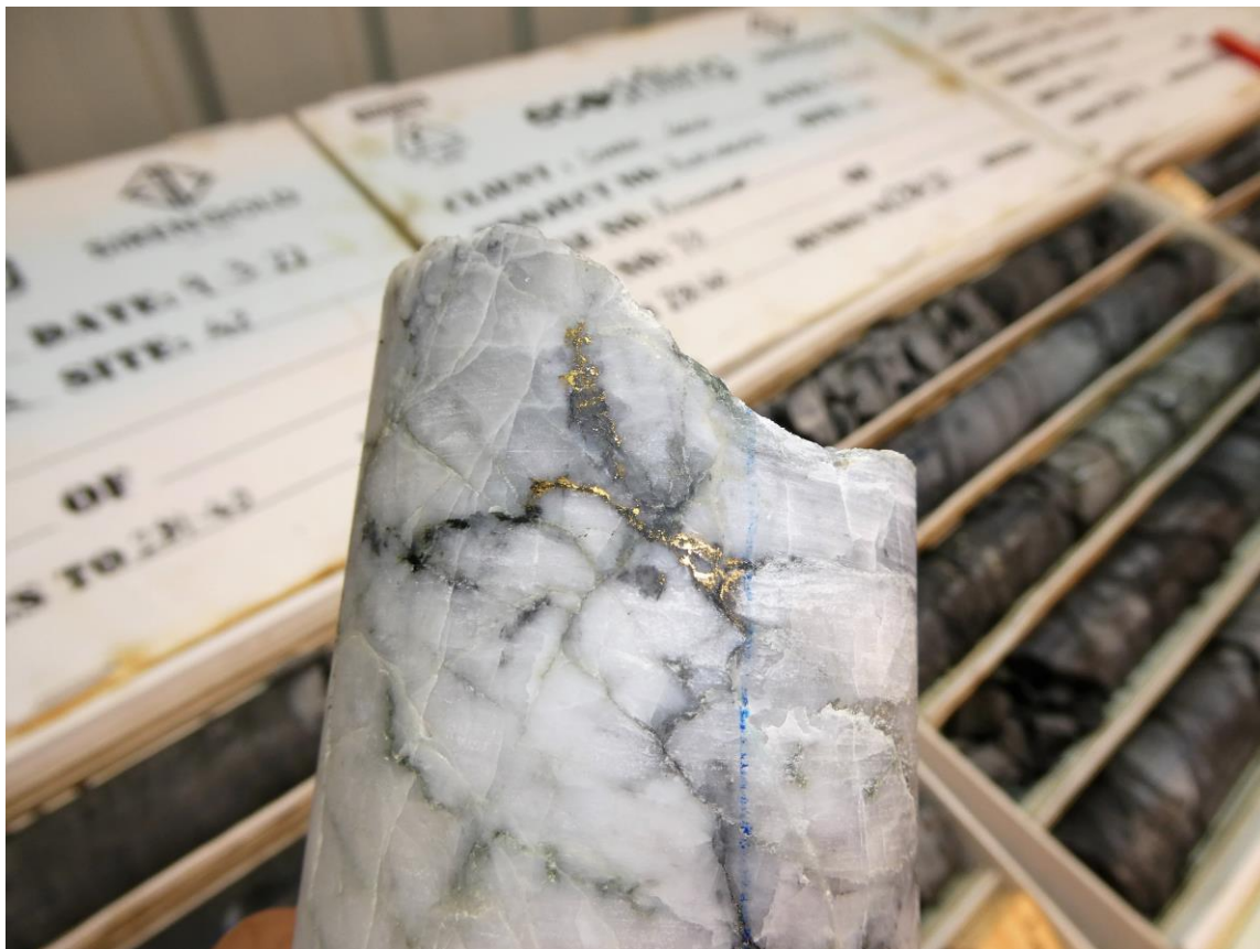
Figure 7. Significant visible gold in a stylolitic seam in hole AX84 at Siren's Alexander River project.
