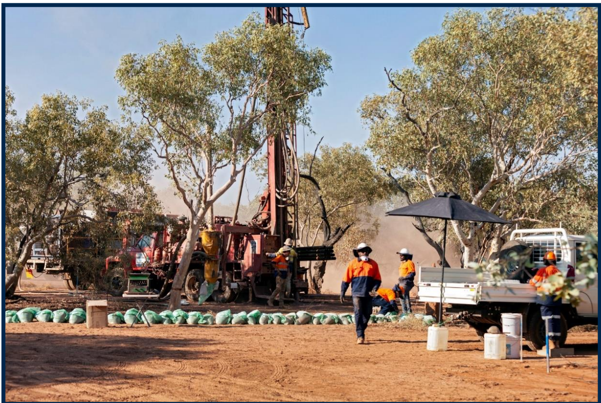
Photo 1: Reverse circulation drill hole (HERC003) in 2021. Note sand cover and lack of surface expression.
