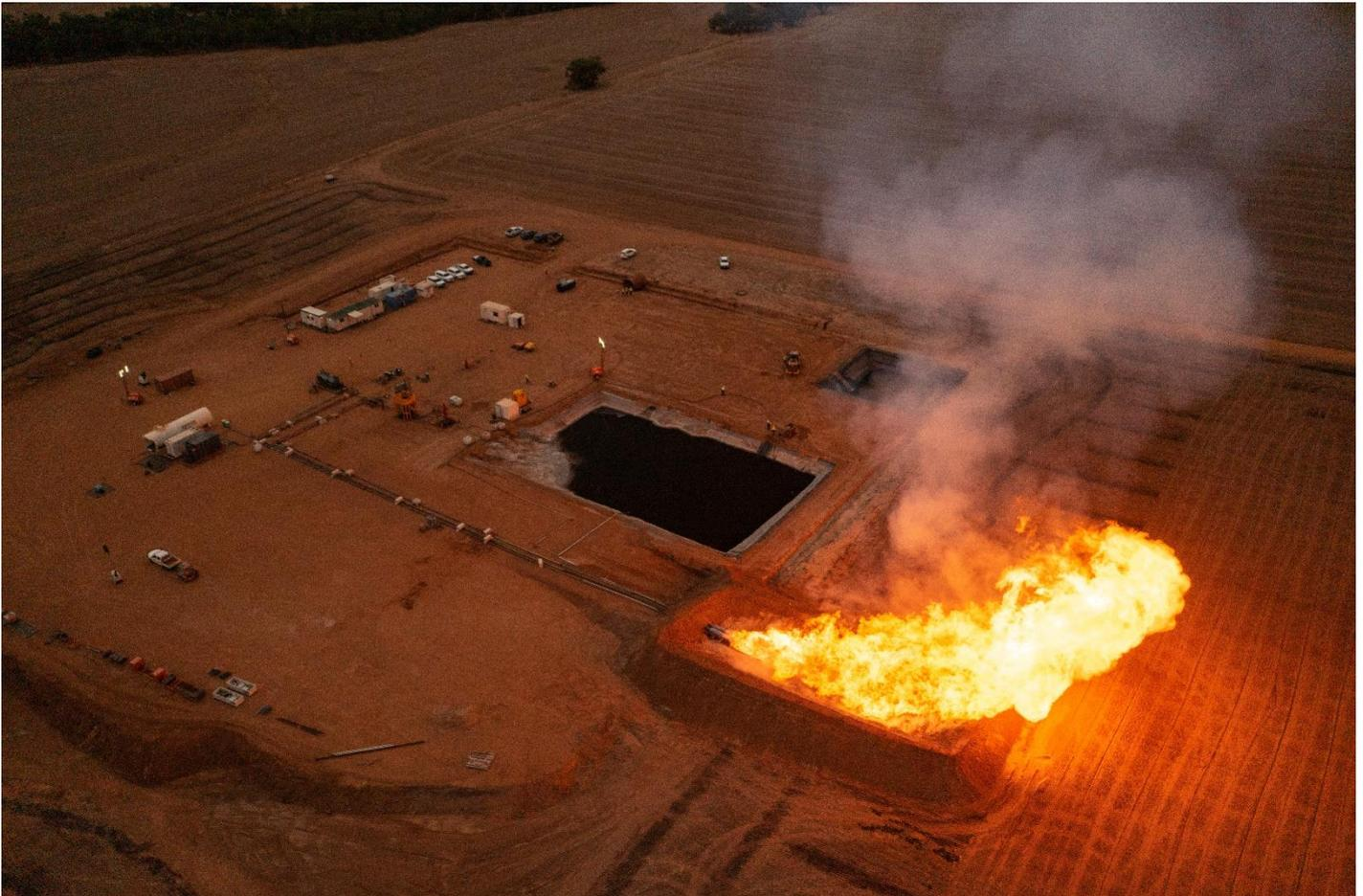
Figure 1 Lockyer Deep 1 gas well flowing at 117 mmscf/day
