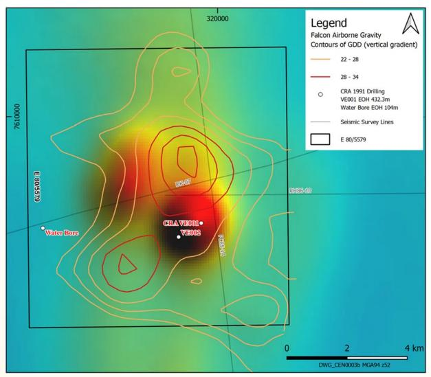
**Figure 2:** Centurion Project summary of open file geophysics. The magnetic image is overlain by airborne gravity contours and seismic lines along with the historical drillhole CRA VE001 (abandoned in the cover sequence above the IOCG target) and the planned VE002 diamond drill hole.
