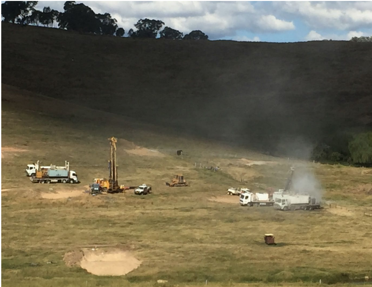
Figure 2 Track mounted Rig (right) drilling hole CAL004 while the Truck mounted Rig setting up to drill. Several drill pads also prepared for drilling.
