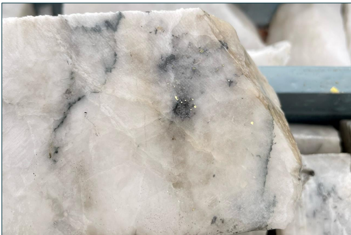
FIGURE 1: VISIBLE GOLD IN 22MBDD002 AT 130M DOWN-HOLE
