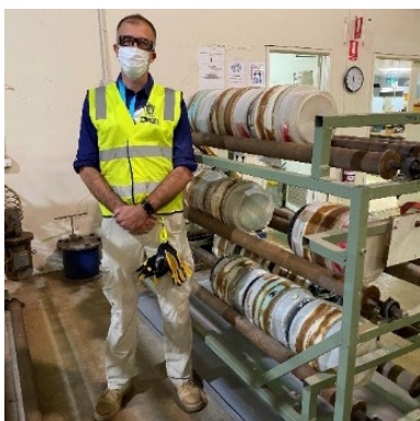
Plate 1 – Managing Director Ian Bamborough checking in on important Apollo Hill Intermittent Bottle Roll Leach Tests at Bureau Veritas's Canningvale Metallurgical Laboratory – December 2021. Crushed rock at various sizes was subjected to a weak cyanide leach solution to extract gold.
