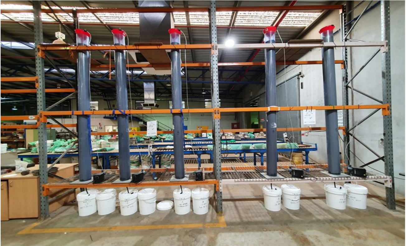
Plate 2 – Apollo Hill Heap Leach column tests underway at Bureau Veritas in Canningvale (March 2022). The tests are being performed across a range of rock types and gold grades and crushing techniques to assess leaching kinetics (speed and efficiency) and scalability.
