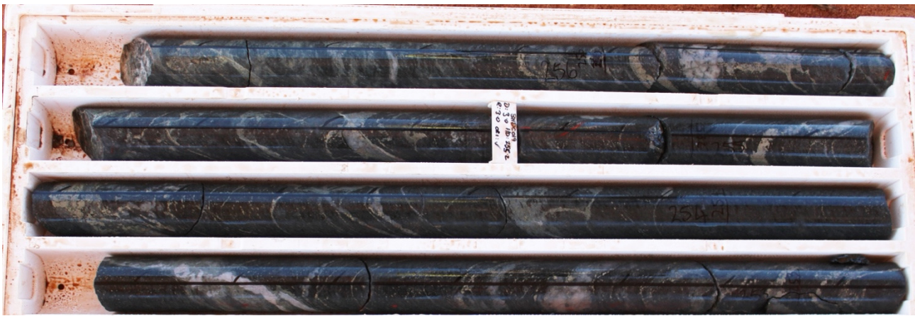
Figure 2: Core Photo BHRCD019 252.8m – 265.5m, showing fine grained basalt with semi massive and disseminated sulphides and magnetite
