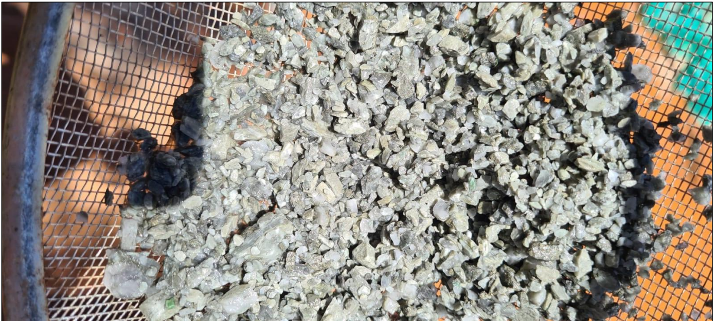
Figure 2 – RC drill chips from hole YRLRC0811 (190-191m) which returned a fire-assay of 19.4g/t Au. Gold mineralisation is hosted within sheared mafic sediments, quartz, fuchsite (green) and sulphides.
