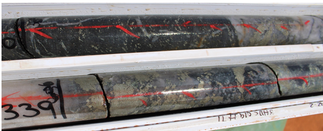
Figure 7: Close-up of BHRCD-019 core from 338.7m – 339m showing quartz veining with massive, blebby and disseminated sulphides comprising pyrite and chalcopyrite, and magnetite (refer to Table 1).
