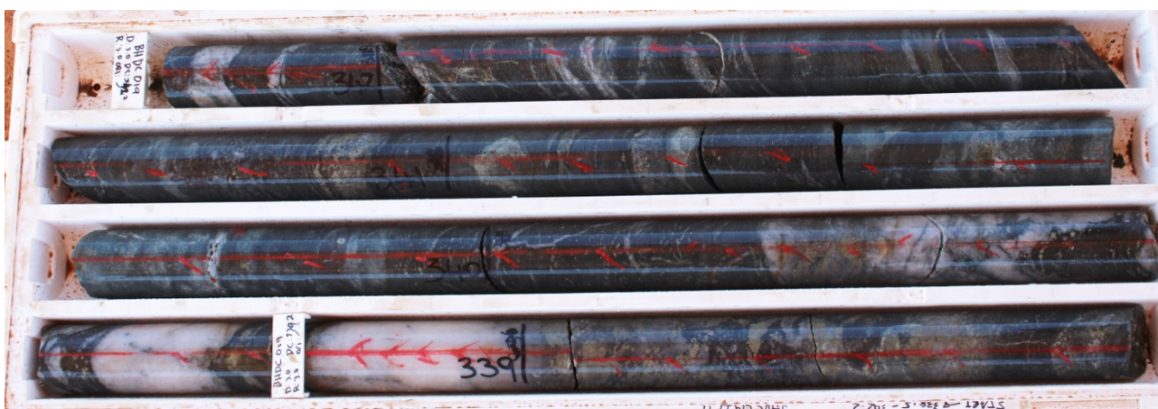
Figure 6. Core Photo BHRCD-019 338.5m – 342.2m downhole, showing Ultramafics with quartz veining and massive and disseminated sulphides, and magnetite.
