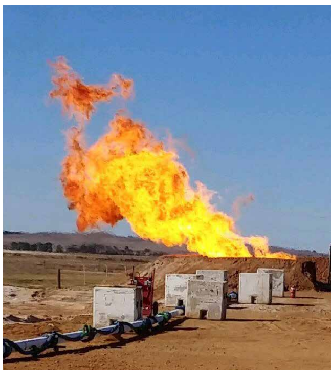
Flow Testing D Sands at Walyering-5
