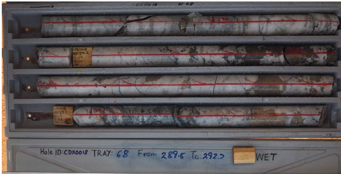
Figure 1. Tray of core from hole CDX0018 showing a portion of the mineralised zone 21.9m at 1.7% TREO including 6.4m at 3.5% TREO from 275.17m down-hole. Massive patches of brown bastnaesite/monazite in carbonatite.
