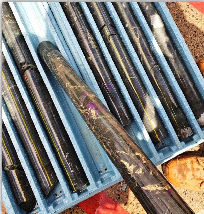
BOD080 – 2m grading 1.01g/t Au, 1.92% Cu from 911m within a zone of 36m grading 0.72g/t Au, 0.40% Cu from 878m – Bornite-chalcopyrite cemented breccia of calc-potassic altered volcanics.
