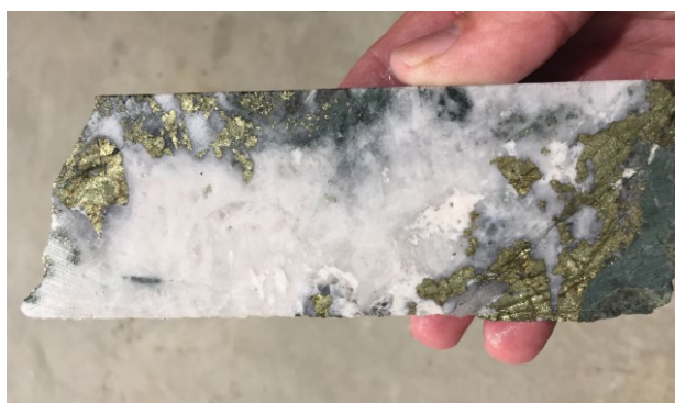
Figure 4: Selected pieces of diamond drill core used for the metallurgical testwork at Mt Chalmers.
