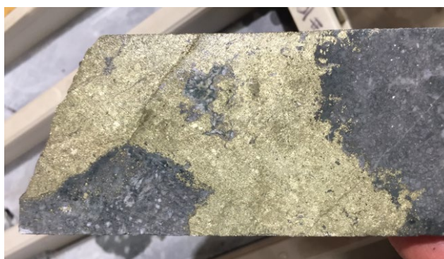
Figure 4: Selected pieces of diamond drill core used for the metallurgical testwork at Mt Chalmers.
