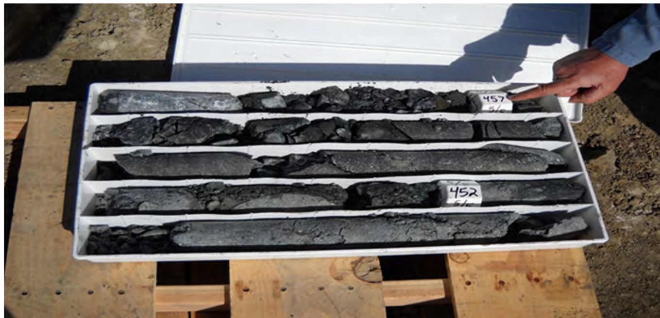
Figure 6: Drill cores showing metasomatic magnetite
