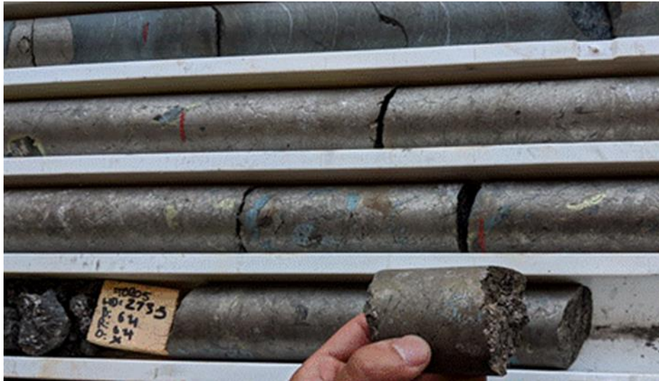
Figure Four | Massive Sulfides in TOR05 from drilling at the Thor Target
