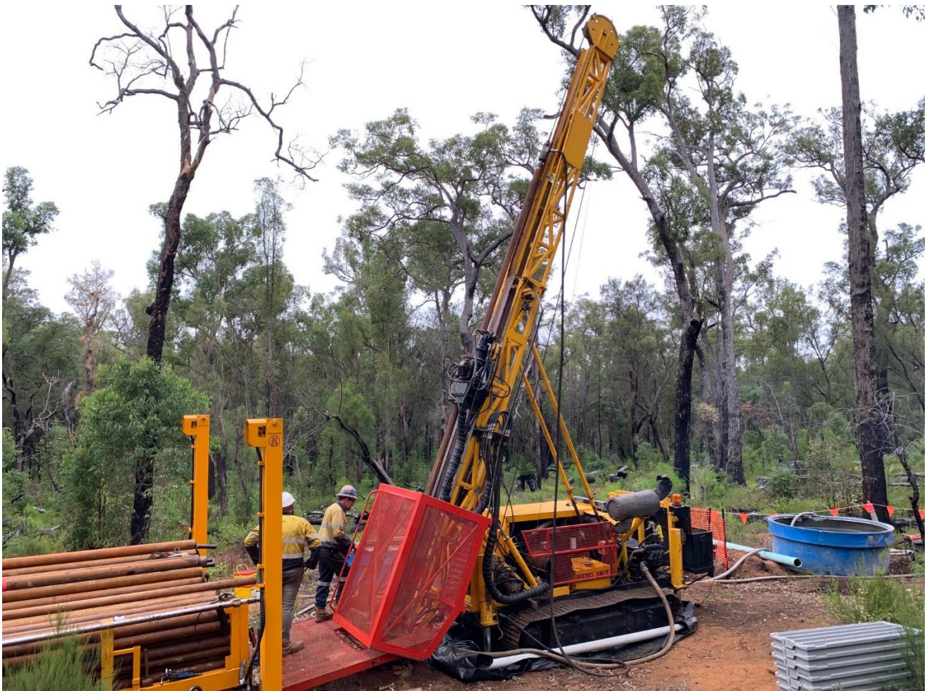
Figure One | Diamond Core Drill Rig drilling the first hole of Chalice's Maiden Drill Program at the South West Project
