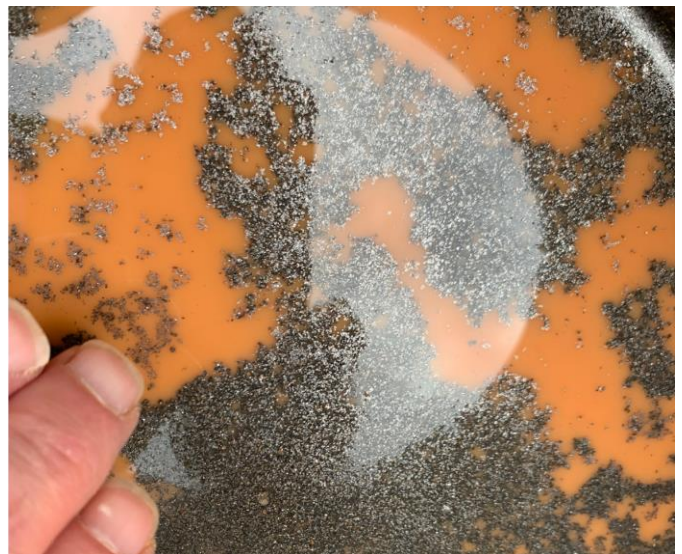
Figures 4 & 5: Very coarse-flake graphite in +600 \mu m sample fraction (L), graphite floating on soaking drill sample (R)
