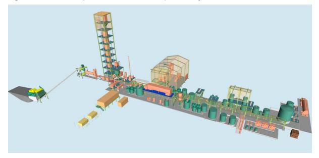
Figure 1 – Mid-stream product demonstration plant design model.
