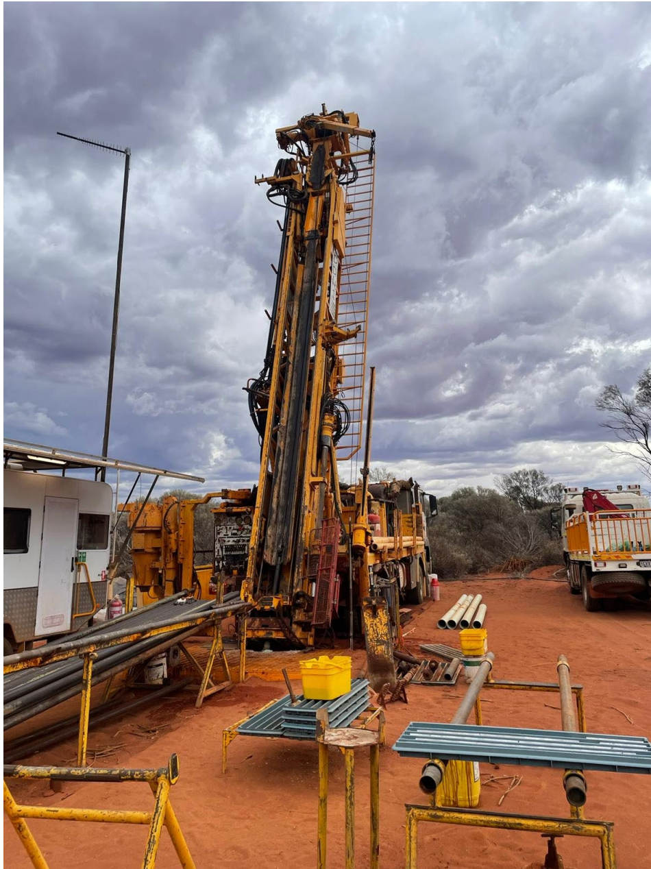
Figure 5 – diamond drilling in progress at Mt Alexander.
