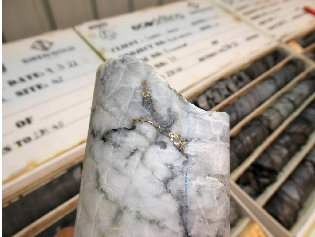
Fig 2. Significant visible gold in Alexander River drillhole AX84 quartz reef in the McVicar West shoot.
