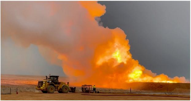
Figure: Lockyer Deep-1 flowing at 117mmscfd
