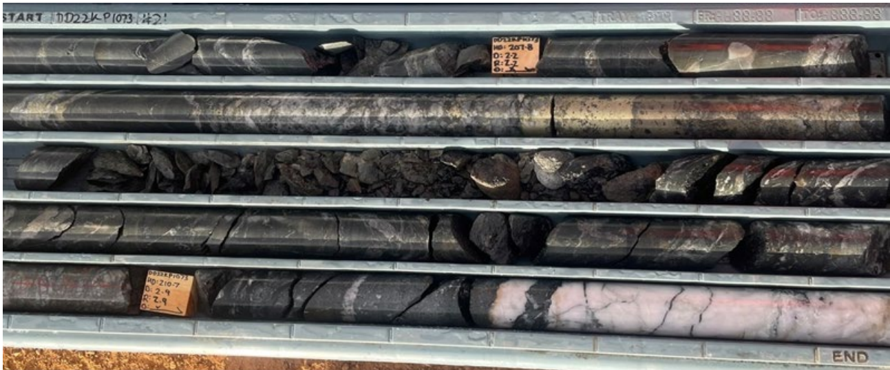
Figure 9: Diamond tail to RC hole RC21KP1073 intersecting the Harbour View South Main lode between 208m and 210.7m. Mineralisation consists of a series of alternating zones with 0.4m quartz + sulphide vein (40% pyrite + chalcopyrite), 0.5m >80% pyrite, pyrrhotite, chalcopyrite followed by 1.1m of intense chlorite-magnetite hosting 10% sulphide stringers.
