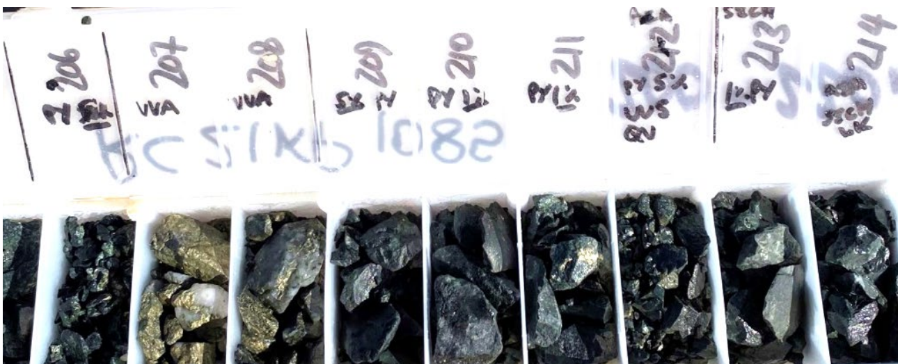
Figure 6: Massive sulphide veining within RC22KP1085 (4m @ 2.54 g/t Au, 1.14% Cu, 11.34 g/t Ag from 205m) between 206-208m with intense chlorite ± magnetite alteration in the footwall with associated sulphide stringer veins. The interval returned and marked the start of the Harbour View Shear.
