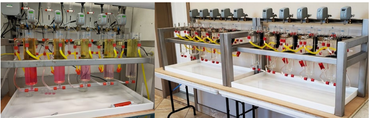
Figure 3: Mixer Settler pilot plant located at Queens University Ionic Liquids Laboratory (QUILL) at QUB.
