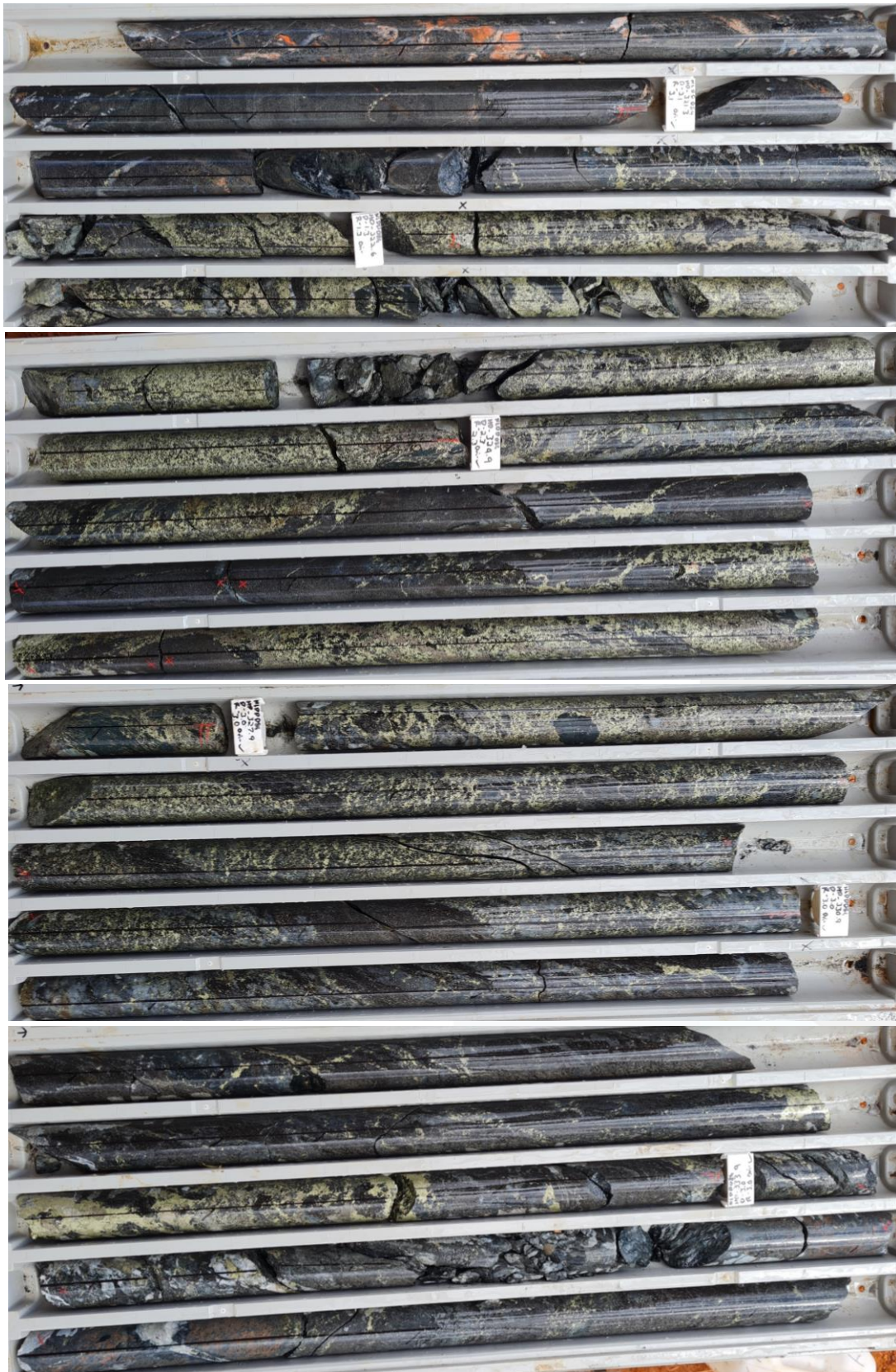
Figure 3. NLDD084 diamond drill core showing high-grade copper mineralisation from 322m to 336m.
