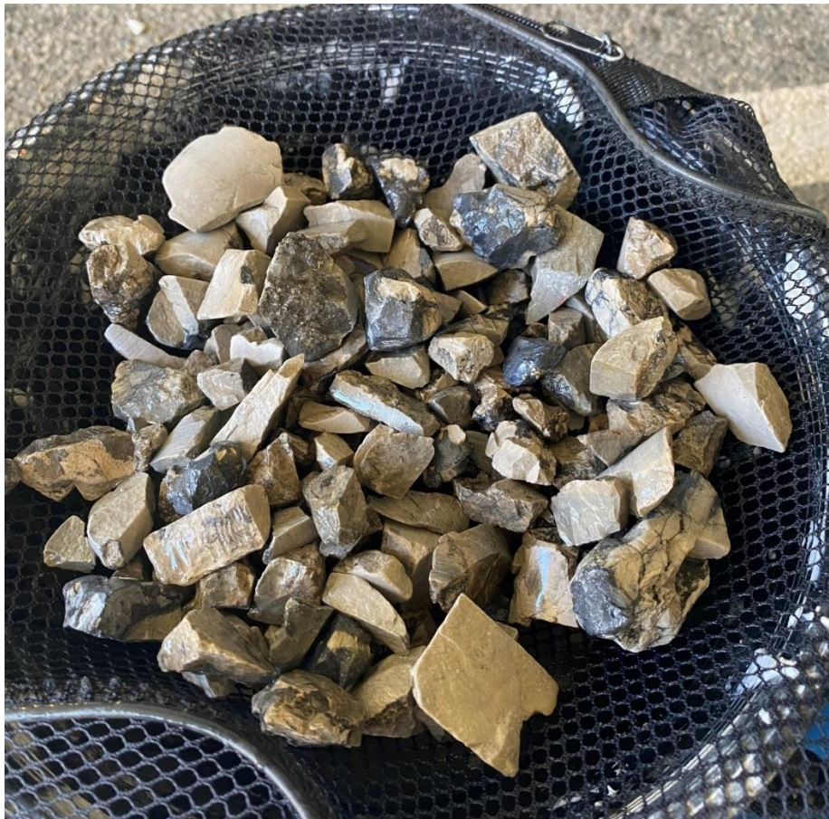
Figure 16: Crushed drill core (10-25mm) from STOR1601D been washed for ore sorting tests
