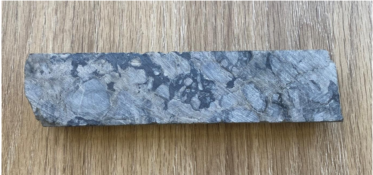
Figure 15: Photo of drill core from STOR1601D from interval 97-101m downhole – average grade 4.16% Cu. Note the semi-massive/breccia chalcocite hosted within dolomite (light grey)
