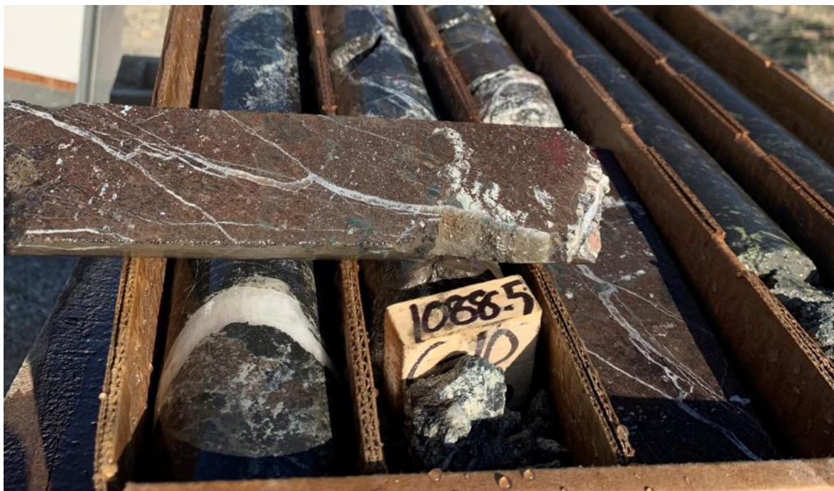
Figure 12: Photo of massive zinc sulphide comprising red-brown sphalerite at approximately 332.8m (1092ft) down hole in drill hole WD22-03. Calcite (calcium carbonate) can be seen as white veins.
