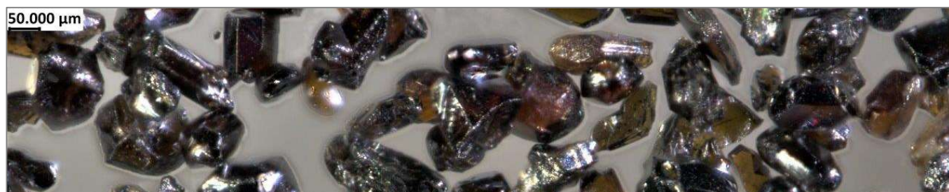
Figure 6: Photomicrograph of high purity rutile product 97.2% TiO 2
