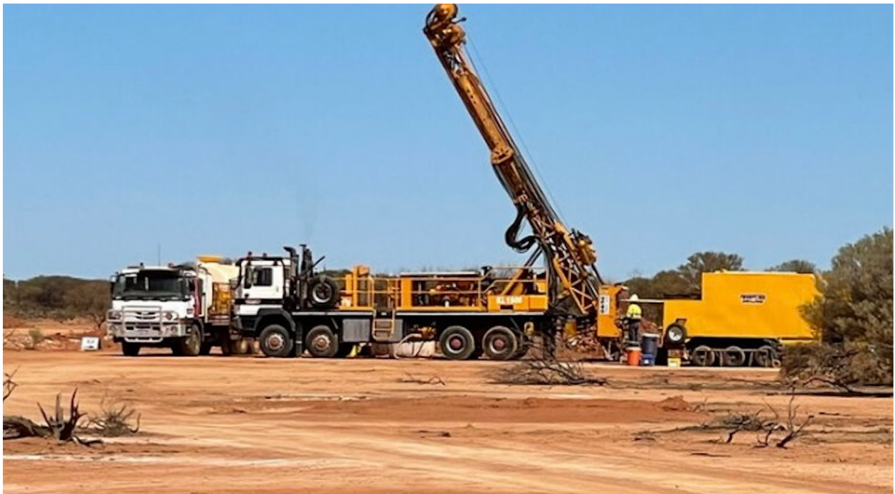
Figure 2. Frontline Drillings KWL 1500 drill rig that has been secured for the program which has the capability to drill total depth of 2500mtrs NQ.
