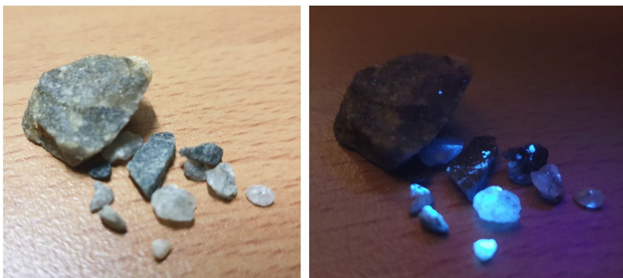
Fig 1 – Monte Cristo Prospect RC drilling rock chips: Natural light vs UV light (scheelite fluorescence)
